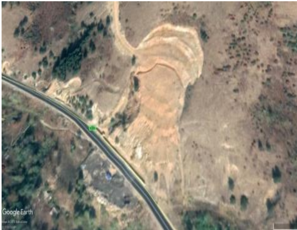
Figure 31. Google Earth snapshot of the Bitola bypass landslides (the smaller area to the left is visible, while the larger landslide is clearly visible in the center)
