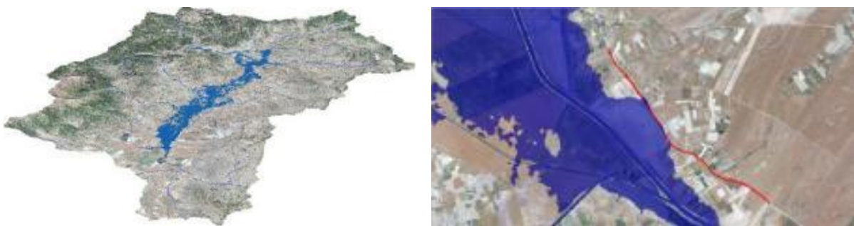
Figure 37. View of the expected flood zone on the Brod-Gneotino route for a defined return period of precipitation
